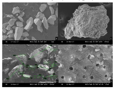
**Figure 3.** (a)Scanning electron microscopy of teeth particles at 1-mm magnification; (b) augmented evaluation of collagenized tooth particles at 200 microns; (c) particle measurements at 200 microns; and (d) dentin tube measurements at 10 microns.
